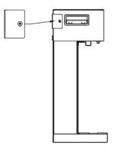
5.3b Choose a solid wall and mark five holes using the holes on the brackets. Drill the marked position using a suitable sized drill bit for the chosen fixings.
