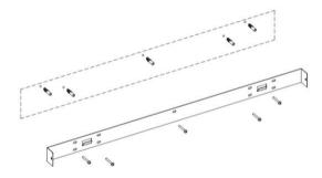
5.3d Use four M4\*8 screws to fix the L brackets on the baseplate of the fire. Hang the fireplace on the brackets and mark the two holes of the L brackets on the wall. Then take down the fireplace. Drill two holes with 8mm drill bit on the marked place. Install two plastic wall plugs. Fix the fireplace on the bracket with two ST4\*8 screws. Use two ST5\*40 screws to fix the L brackets on the wall.
