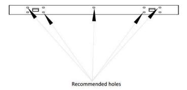
5.3c Tap the plastic wall plug into the five holes. Then use five ST5\*40 screws to fix the brackets on the wall.
